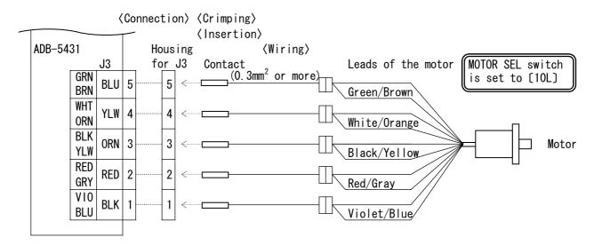
■Color indications for the motor crimping J3 represent colors of the leads of the motor.
