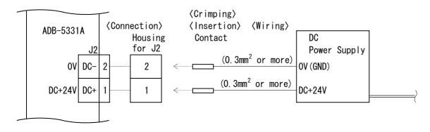
●Do not power ON/OFF by the relay etc. in the output side of the DC power supply.
