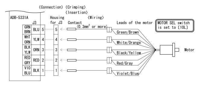
■Color indications for the motor crimping J3 represent colors of the leads of the motor.
