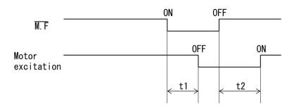
$t1 \le 5ms$  (t1: Time required for the motor output current to be shut off.)
