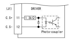
Step angle division is switched to 20 divisions of the basic angle with the photo-coupler ON.
