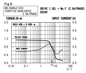
Fig. 7 DB-2640v2/U16 P-PMSA-U42D3M(U42D3MD) DRIVE I. SEL = No. 5 (0. 8A/PHASE) DC24V TORQUE (N·m) INPUT CURRENT (A) 0.5 5.0 HOLD 40% = 0.14N · m 0.4 4.0 PULLOUT TORQUE 0.3 3.0 0.2 2.0 0.1 1.0 0.0 0.0 fs<sub>10</sub> 0.01 0.1 1 100  $(s^{-1})$
