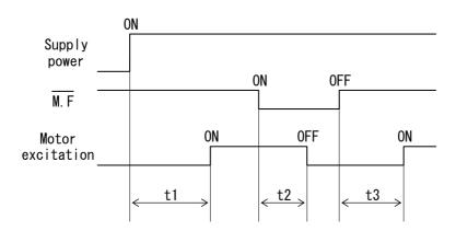
$t1 \le 300$ ms (t1: Time required for the motor to be enabled.)
