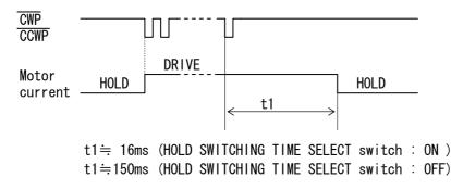
Inputting drive pulse causes the current output to the motor to change from HOLD CURRENT to DRIVE CURRENT, which returns to HOLD CURRENT in about "t1".
