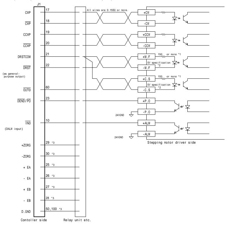
\*1 If the current limiting resistor on the driver side is less than 150 , externally add resistor so that the total resistor value becomes 150 or more.
