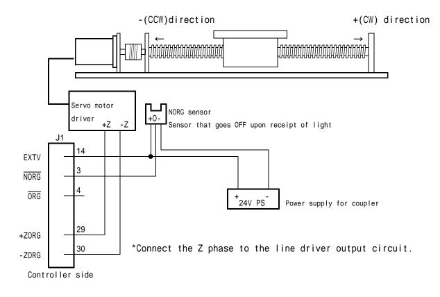
When using the Z-phase signal of an encoder
