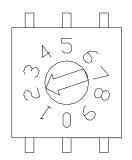
The S1 setting is validated after power-on. Set the switch with power off, and turn it on after changing the setting.
