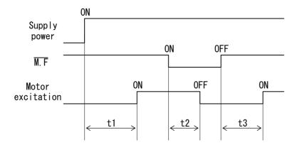
$t1 \leq 300 ms$  (t1: Time required for the motor to be enabled.)
