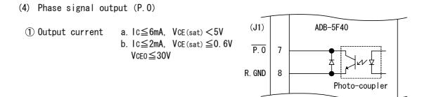
● In case of the excitation home position, the signal is output. (photo-coupler ON)
