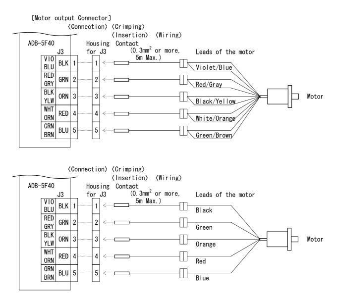
●Color indications for the motor crimping J3 represent colors of the leads of the motor.
