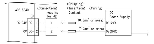
●Do not power ON/OFF by the relay etc. in the output side of the DC power supply.
