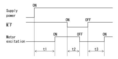
$t1 \le 1.5s$  (t1: Time required for the motor to be enabled.)
