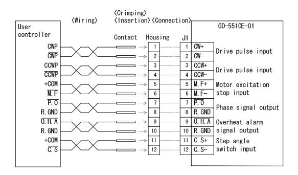
lacktriangle Use a signal cable of AWG26 (0.15mm<sup>2</sup>) or more in diameter.
